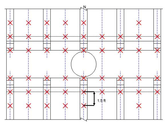
Figure 5.34: Deck Reinforcement Strain Gauge Layout
