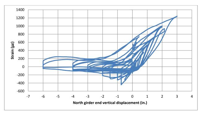
Figure 6.51: Strain History on Unstressed Strand in Exterior Girder-to-Cap Improved Connection
