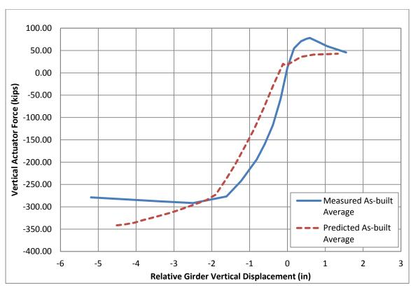
Figure 6.45: Predicted vs. Measured Total Force vs. Relative Displacement for As-built Connection
