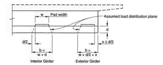
Figure B.8. Distribution Plane Layout (Caltrans, Bridge Design Specifications, 2003)
