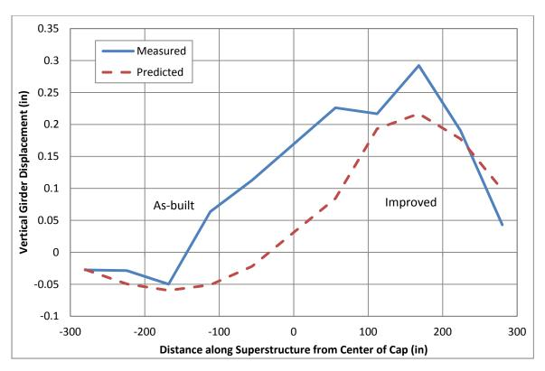
Figure 6.9: Center Girder Vertical Displacements at  $\mu_{\Delta}$  = +8
