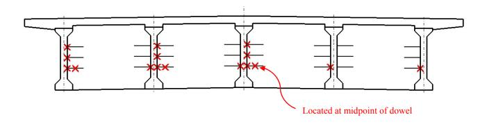
Figure 5.31: Girder-to-Diaphragm Dowel Strain Gauge Locations
