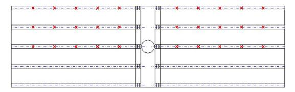
Figure 5.38: Locations of Vertical Displacement Devices along the Girder Length During Phase 1 of Testing
