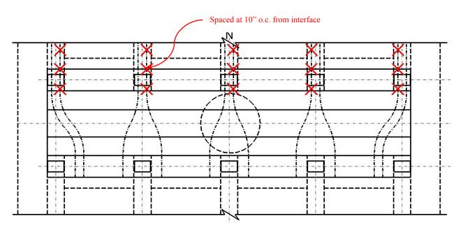
Figure 5.32: Improved Connection Strand Strain Gauge Locations
