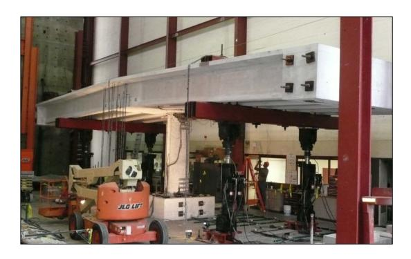
Figure 6.36: Displaced Test Unit at -6 in. of Displacement
