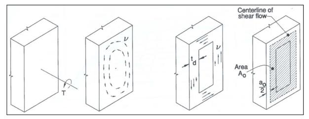
Figure 2.14: Torsion Hollow Tube Analogy (Collins & Mitchell, 1991)
