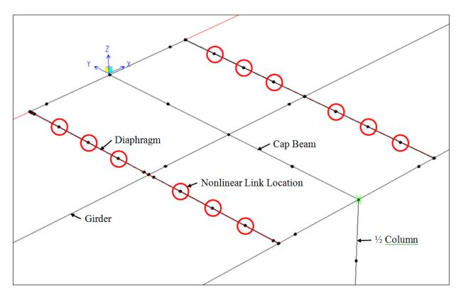
Figure 4.23: Locations of Grillage Model Nonlinear Link Elements Used to Model Cap-to-Diaphragm Reinforcement
