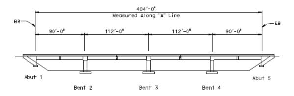
Figure 3.1 Prototype Bridge Elevation View
