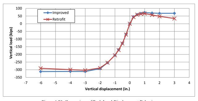
Figure 6.39: Comparison of Peak Load-Displacement Behavior
