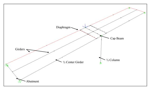
Figure 4.8: Test Unit Grillage Model
