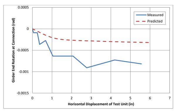
Figure 6.16: Center Girder Improved Connection Girder Rotation/Gap Closing
