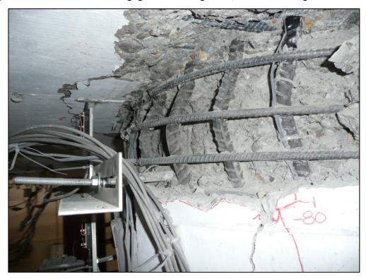
Figure 6.3: Buckling in the Top Column Hinge on the North Side at  $\mu_{\Delta}\!\!=\!\!10$
