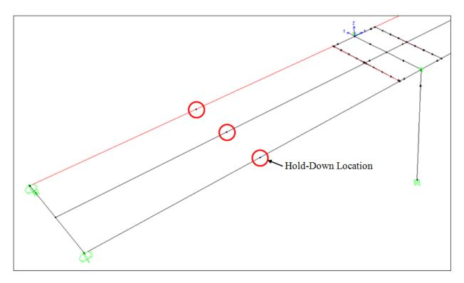
Figure 4.27: Grillage Model Hold-Down Node Locations
