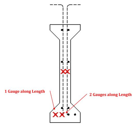
Figure 5.28: Girder Cross-Section Strain Gauge Locations
