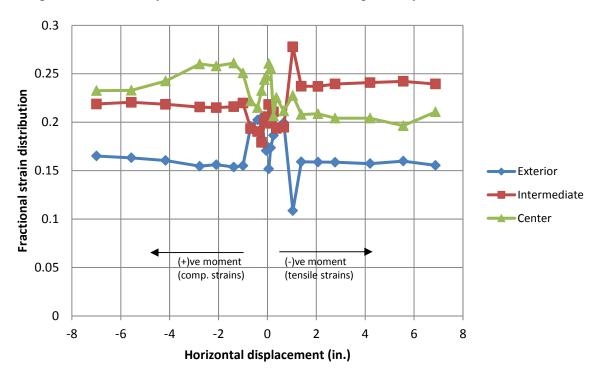
Figure 6.24: Contribution of Moment Resistance by Girders on the Improved Connection Side 1.5 feet from the Diaphragm Edge
