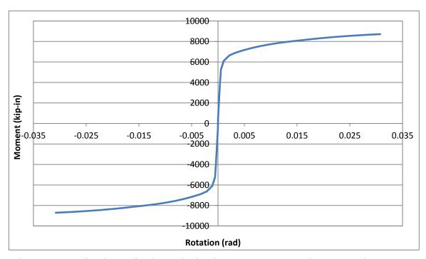
Figure 4.13: Predicted Top of Column Plastic Hinge Moment vs. Rotation Monotonic Response
