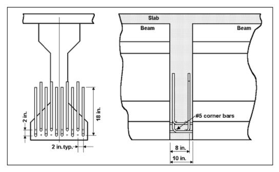
Figure 2.4. NCHRP Bent Strand Specimen (Miller et. al., 2004)
