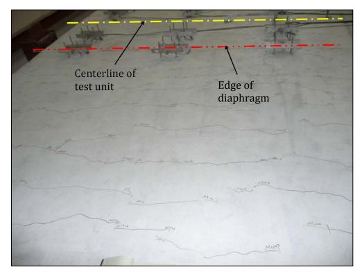
Figure 6.4: Distribution of Flexural Cracking on the Top Side of the Deck at  $\mu_{\Delta}$ =+10
