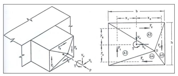
Figure 2.17: Torsion Shear-Friction Model (Priestley et. al., 1996)
