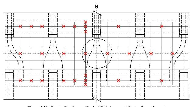
Figure 5.23: Cap-to-Diaphragm Hooked Reinforcement Strain Gauge Layout
