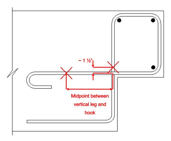
Figure 5.30: Girder Dapped End Detail Strain Gauge Locations
