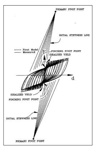
Figure 2.11: Pivot Model Observations (Dowell et. al., 1998)
