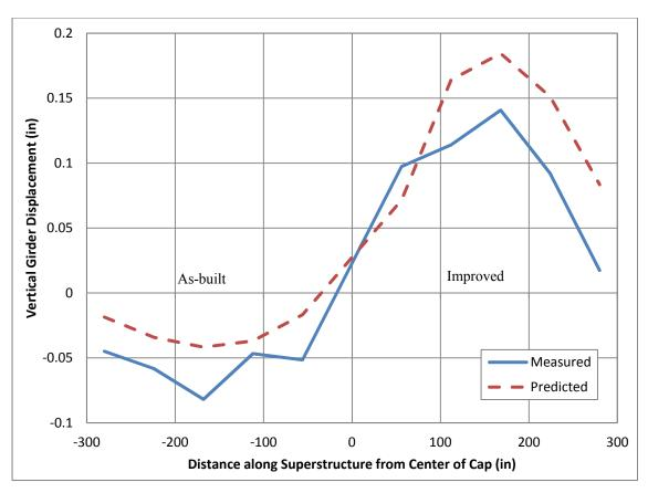
Figure 6.7: Center Girder Vertical Displacements at  $\mu_{\Delta} = +3$
