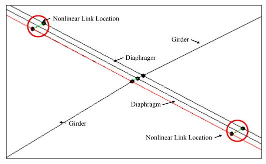
Figure 4.25: Grillage Model Improved Connection Nonlinear Link Location
