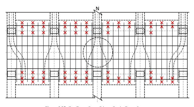
Figure 5.27: Cap Beam Outer Stirrup Strain Gauge Layout
