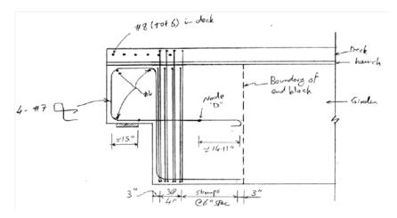
Figure B.16. Dapped End Region Reinforcement Layout
