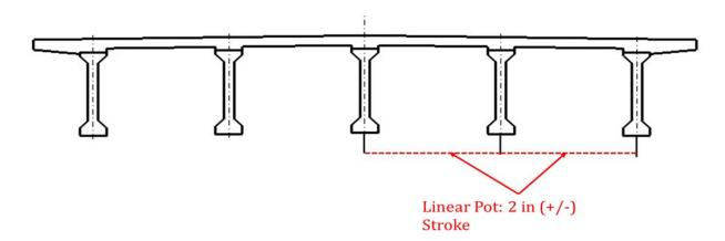
Figure 5.44: Lateral Displacement between Girders Device Locations
