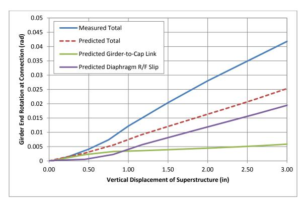
Figure 6.46: Positive Vertical Displacement vs. Center As-built Girder Rotation
