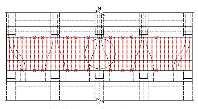
Figure 5.25: Cap Beam Inner Stirrup Strain Gauge Layout
