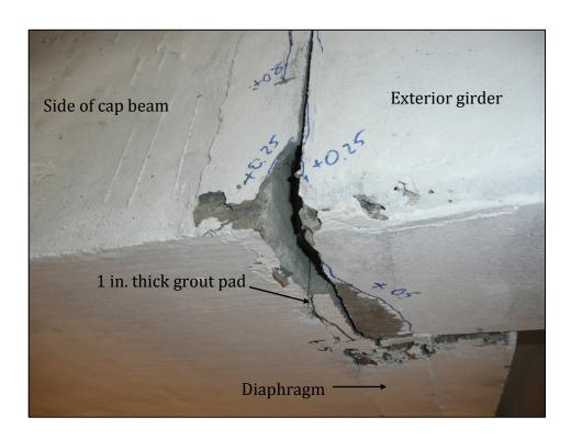
Figure 6.31: Partially Spalled Grout Pad at Girder-to-Cap Interface on the As-built Connection Side at +0.75 in. Displacement
