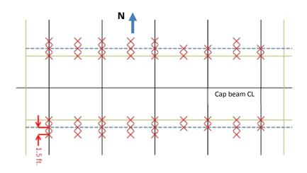
Figure 6.54: Deck Reinforcement Strain Gauges
