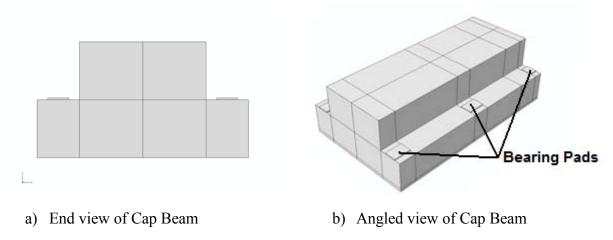
Figure 4.5. Views of modeled Cap Beam
