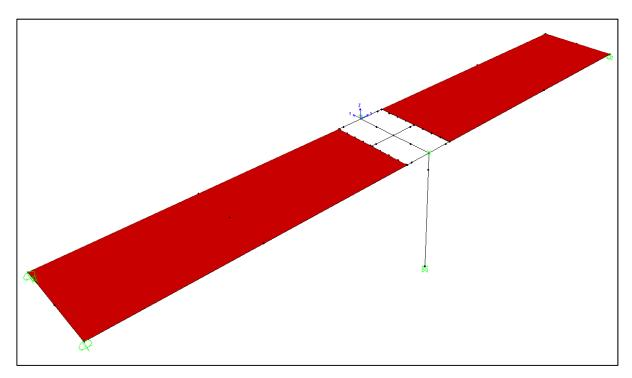
Figure 4.10: Grillage Model after Adding the Area Deck Elements
