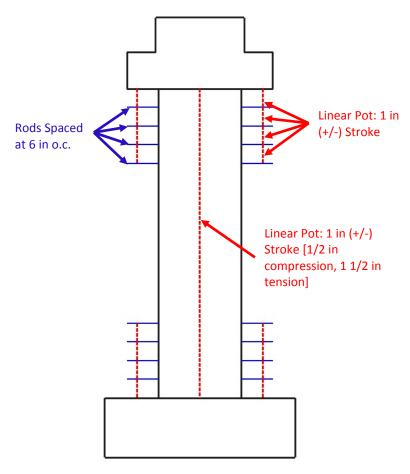
Figure 5.40: Column Curvature and Growth Device Locations
