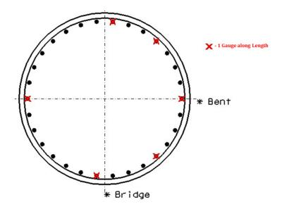
Figure 5.21: Bottom of Column Longitudinal Reinforcement Gauges
