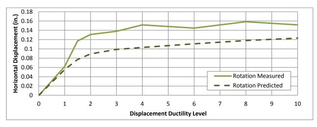
(c) Displacement due to plastic hinge rotation
