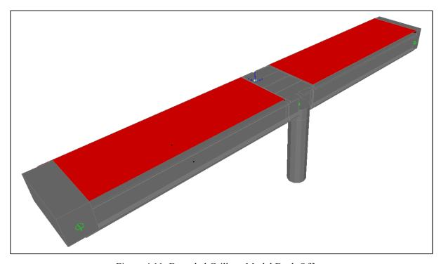
Figure 4.11: Extruded Grillage Model Deck Offset
