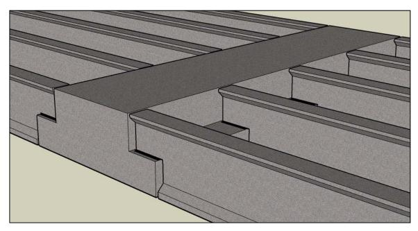
Figure 1.3: Inverted-T Bent Cap
