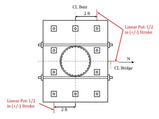
Figure 5.46: Footing Displacement Device Locations
