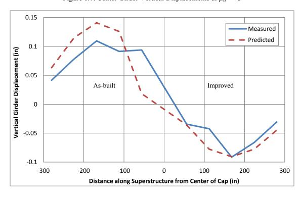
Figure 6.8: Center Girder Vertical Displacements at  $\mu_{\Delta}$  = -3
