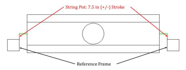
Figure 5.36: Plan View of Horizontal Cap Beam Displacement Devices
