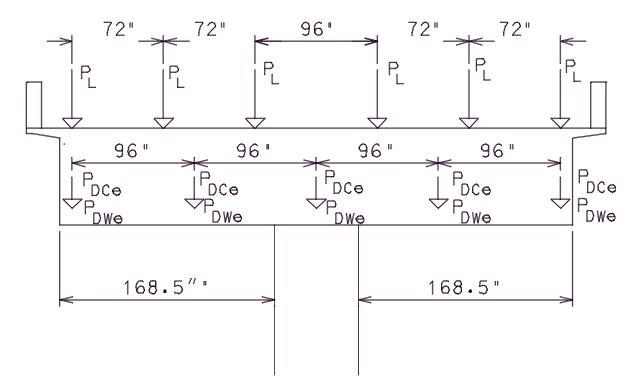
Figure B.3. Load layout on cap beam
