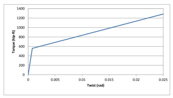
Figure 4.17: Predicted Inverted-T Cap Beam Torque-Twist Response
