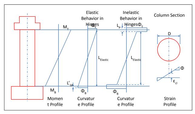
Figure 5.49: Estimating Column Growth in the Vertical Direction
