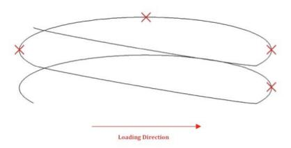
Figure 5.19: Typical Column Spiral Gauge Location
