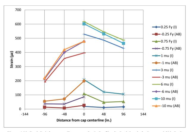
Figure 6.22: Deck Reinforcement Transverse Strain Profiles for Peak Loads for Improved Side Push
