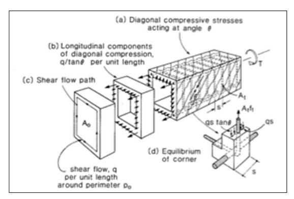
Figure 2.15: Torsional Behavior Post-Cracking (Collins & Mitchell, 1991)
