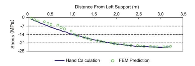
Figure 2.6. Compressive stress in top fiber of the beam (Biggs et. al., 2000)
