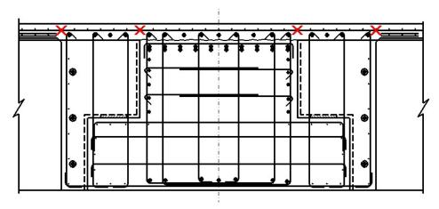
Figure 5.33: Deck Reinforcement Strain Gauge Locations
