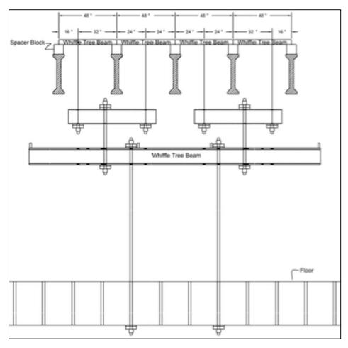
Figure 5.59: Whiffle Tree Arrangement used to Impose Additional Vertical Loads to the Test Unit during
