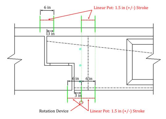
Figure 5.43: Girder-to-Cap Beam Connection Instrumentation Scheme
