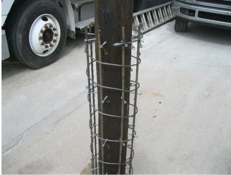
Figure 11-4 Pile jacket half-scale model
