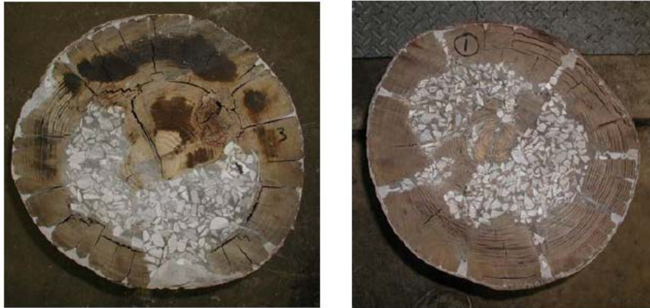
Figure 3-17 Cross-sections of epoxy- and aggregate-repaired piles
