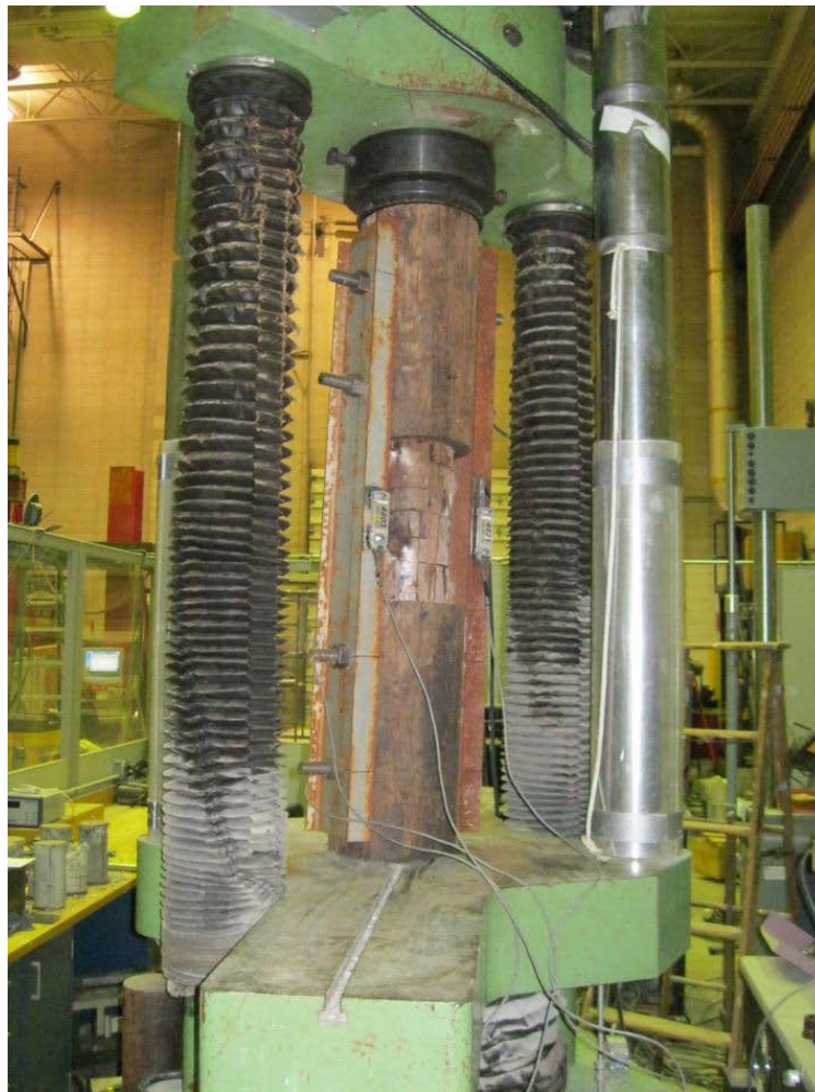
Figure 7-3 Sistered pile with channels and through bolts
