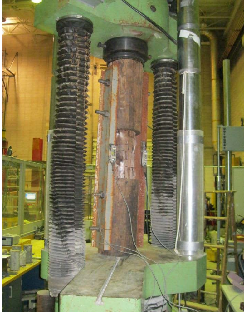
Figure 3-7 Pile strengthened with steel sisters
