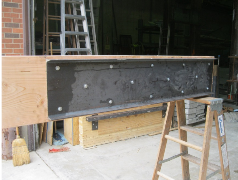
Figure 11-2 Stringer sister half-scale model
