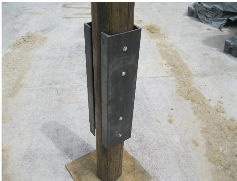
Figure 11-3 Pile channel reinforcement half-scale model
