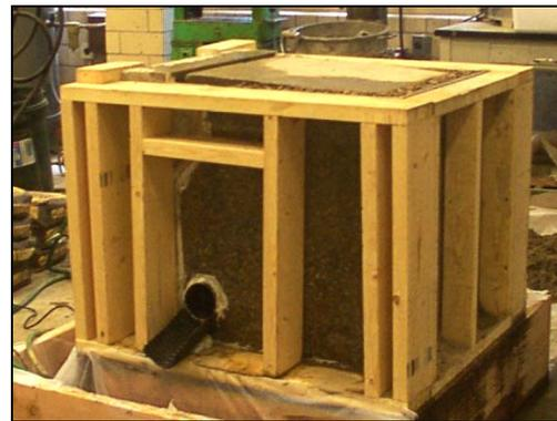
**Figure 9. Using porous fill material behind the abutment**
