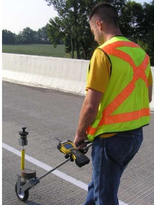
b. 360 degree prism and mono-wheel cart
