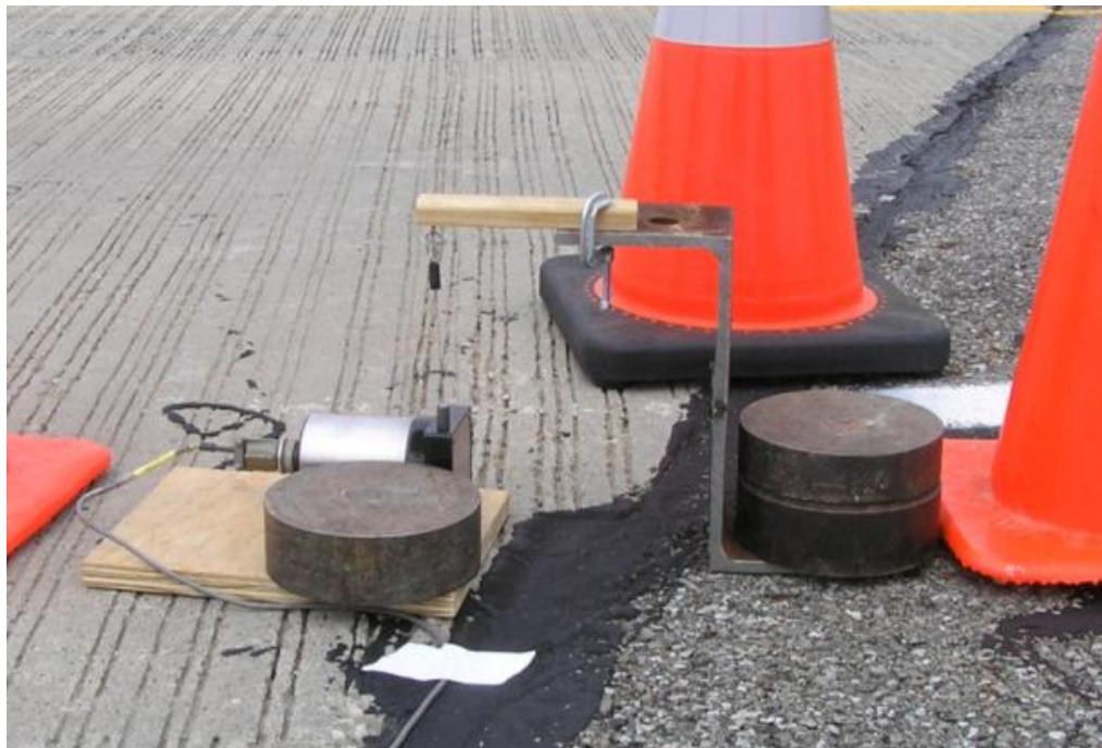
Figure 5.5. Displacement transducer at approach-pavement joint
