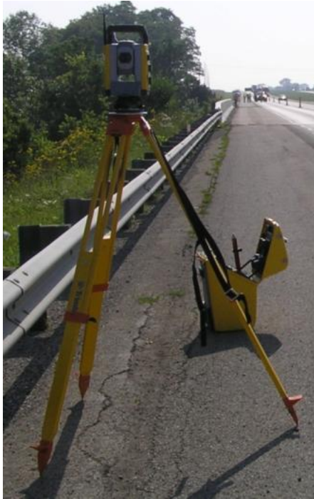
a. Trimble SPS930 laser guided total station
