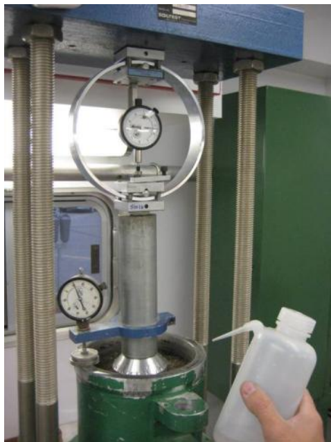
Figure 6.1. Laboratory evaluation of the collapse potential of the backfill materials
