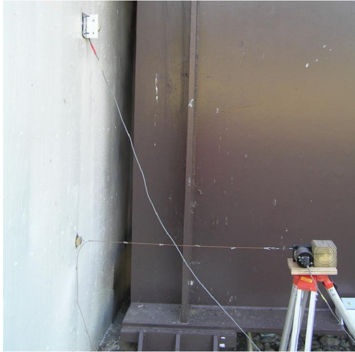
Figure 5.6. Abutment horizontal translation and rotation monitoring
