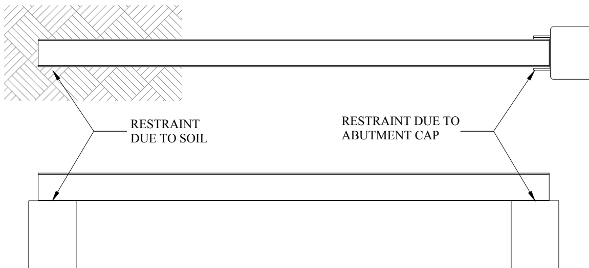
Figure 2.34. Correlation of field conditions to the laboratory set-up
