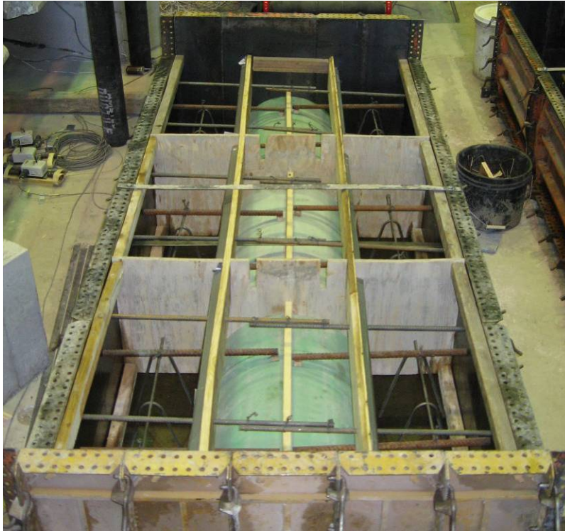
Figure 2.23. Completed formwork for Type 3 Connection
