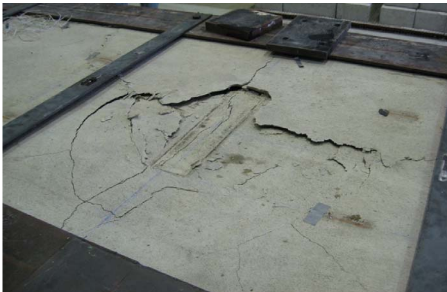
Figure 3.22. Failed abutment backwall specimen
