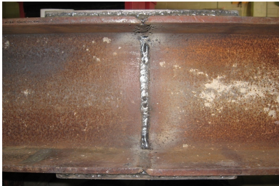
Figure 3.20. Repaired H-pile splice
