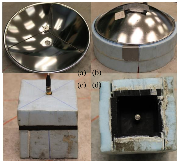
Figure 2.11. Equipment used to reduce noise: parabolic reflector with microphone mount (upper left), parabolic reflector with foam annulus(upper right) and rubber and foam sound isolation enclosure (lower left and lower right).
