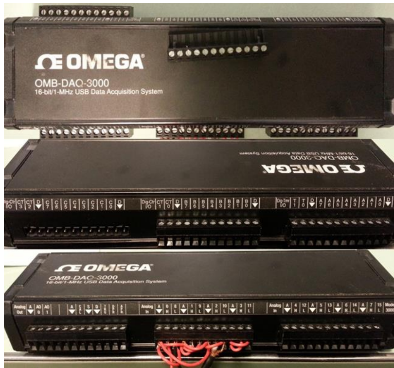
Figure 2.8. Omega OMB-DAQ-3000 1-MHz, 16-bit data acquisition system.
