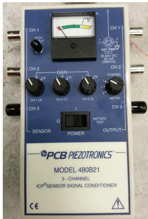
Figure 2.7. PCB model 480B21 battery-powered sensor signal conditioner.
