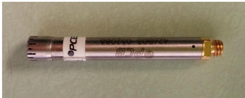
Figure 2.5. PCB model 378C01 microphone used as air-coupled sensor.
