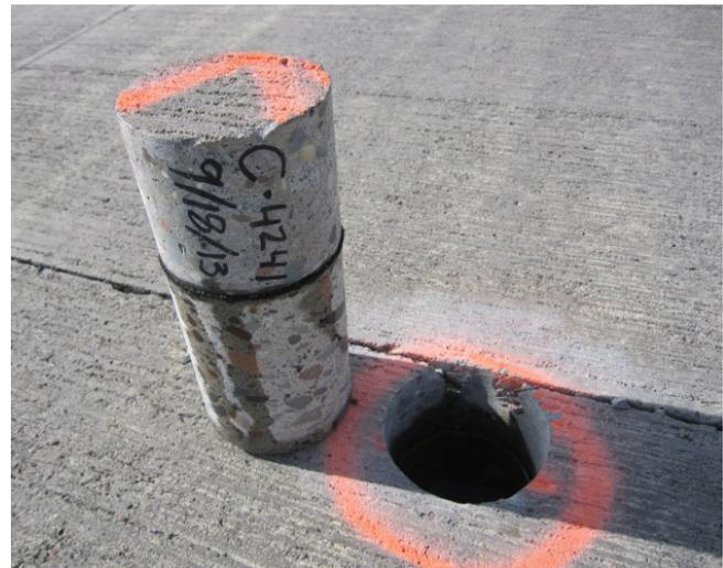
*Sample core retrieved in 2013 showing the relationship to Joint 4241 Cell 505 with its fabric bond-breaker*
