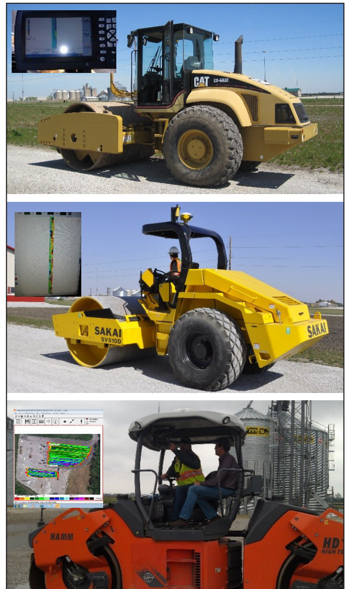
Figure 1. (top to bottom) Caterpillar CS683 smooth drum roller, Sakai SV610D smooth drum roller, and Hamm HD120VV double smooth drum roller (courtesy of Hamm-Writgen Group) with system displays (insets)
