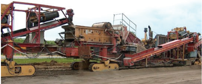
Figure 3.2. Mobile on-site crushing equipment
