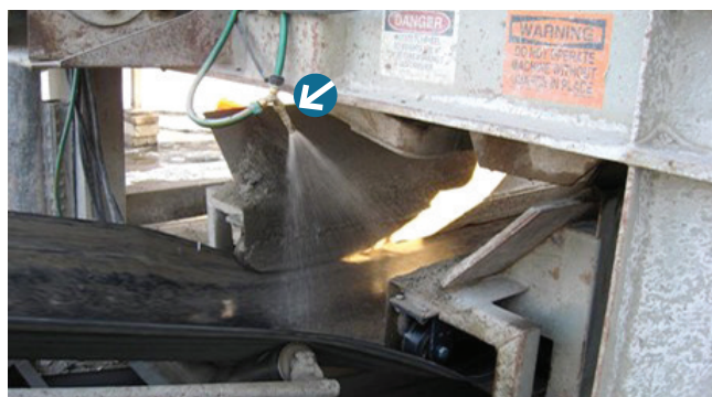
Figure 7.5. Spray nozzle for dust control on aggregate conveyor
