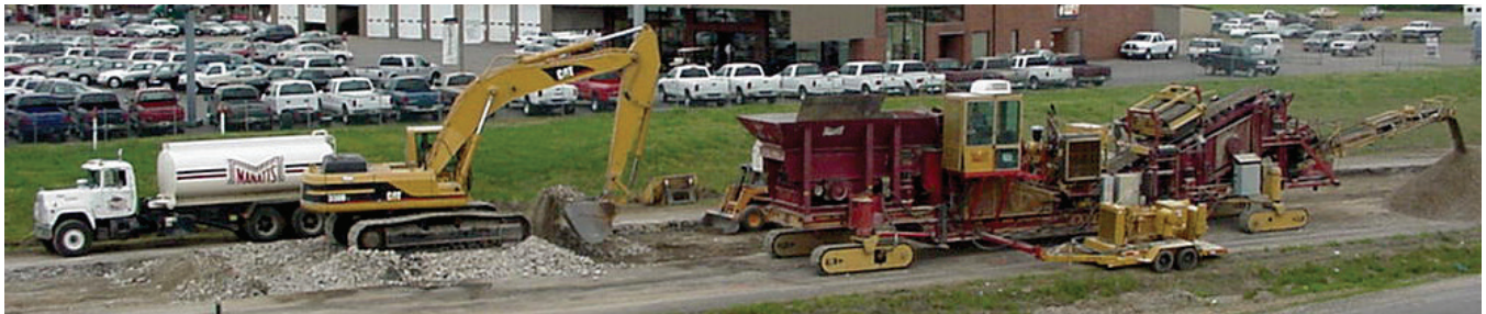
Figure 1.2. Typical on-site mobile concrete pavement recycling operation
