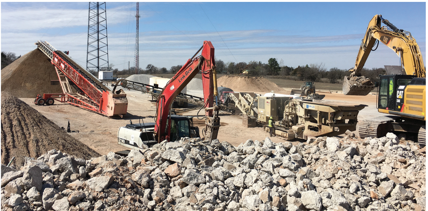
Figure 3.3. Crushing and sizing of source concrete at an on-site stationary plant
