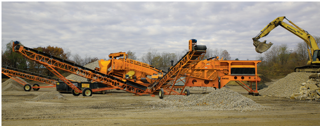
Figure 2.1. Mobile aggregate processing plant
