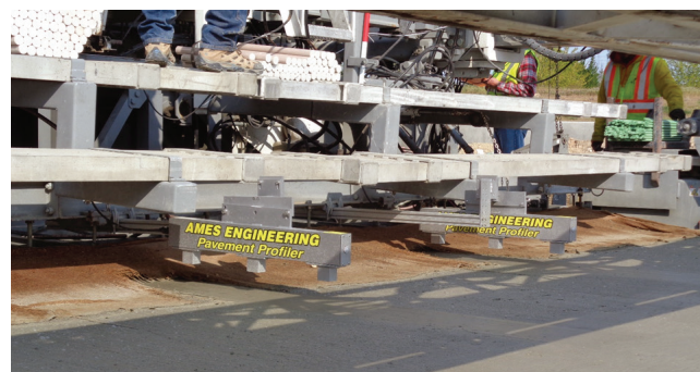
Figure 8-26. Real-time smoothness device mounted to the back of a paver
