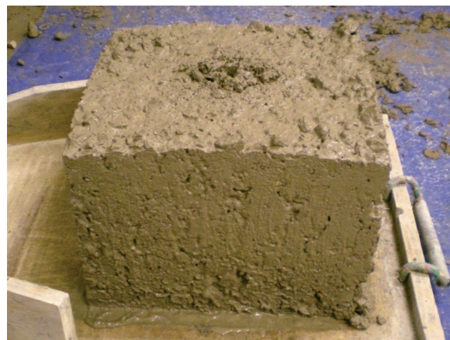
Figure 6-3. Box test sample after the forms are removed
