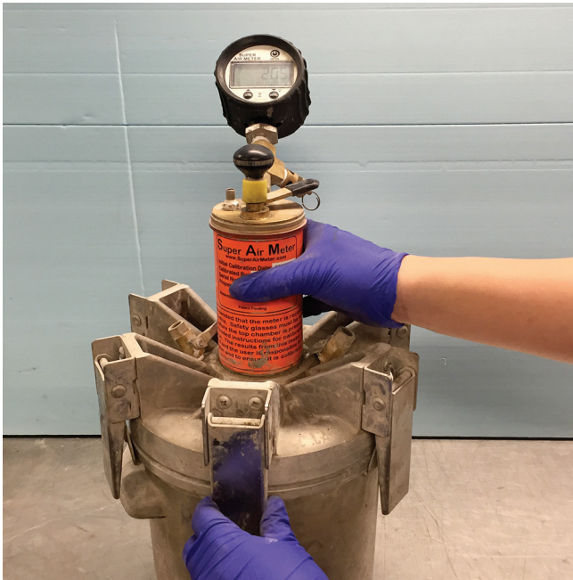
Figure 9-6. Super air meter
