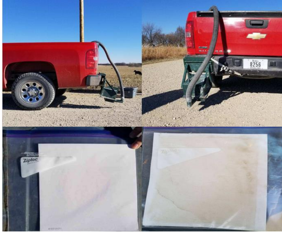
Figure 21. Dustmeter setup, top, and dust production measurement paper, bottom
