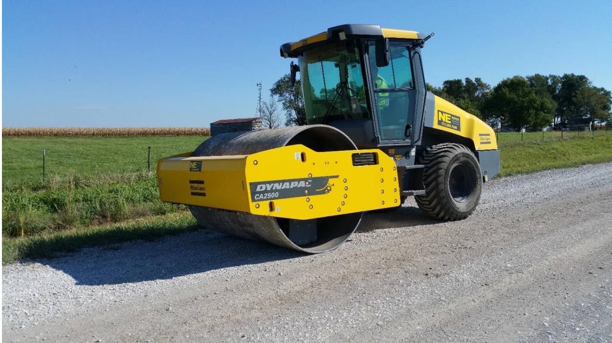
Figure A.2. Drum roller used to compact the shaped surfaces
