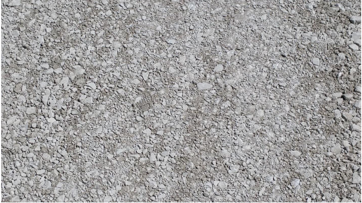
Figure A.6. Compacted surface of the first section after construction
