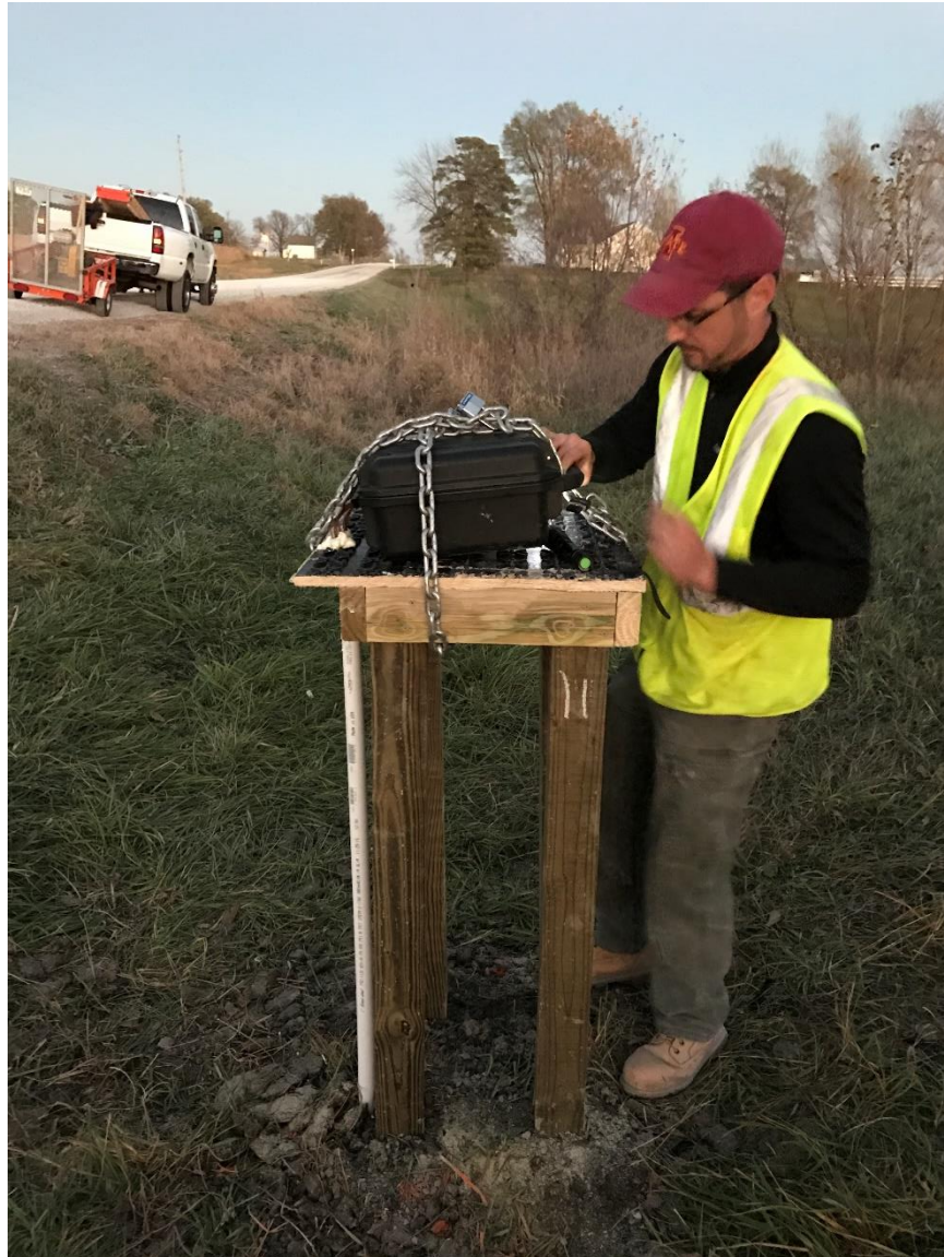
Figure E.7. Locking the data loggers
