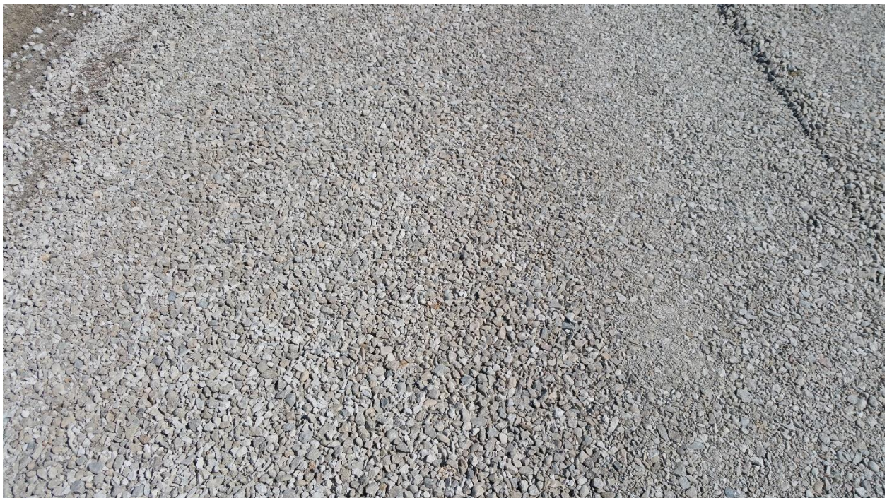
Figure A.27. Compacted surface of 70% BFL Class A + 30% CRG Clean
