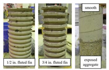
Four surface conditions used to evaluate socket connection performance
