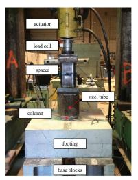
Test setup for socket connection tests
