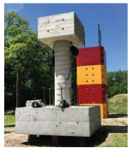
Assembled half-scale test unit for outdoor system test
