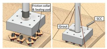
Construction of column/footing/pile system
