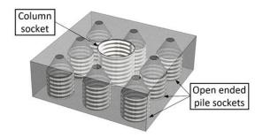
Precast pile cap with preformed sockets
