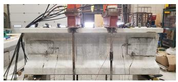
Patched beam specimen instrumented for the four-point bending test
