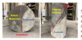
Specimens for splitting tensile strength test (left) and slant shear strength test (right)
