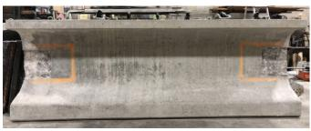
Beam specimen with artificial damage on both ends
