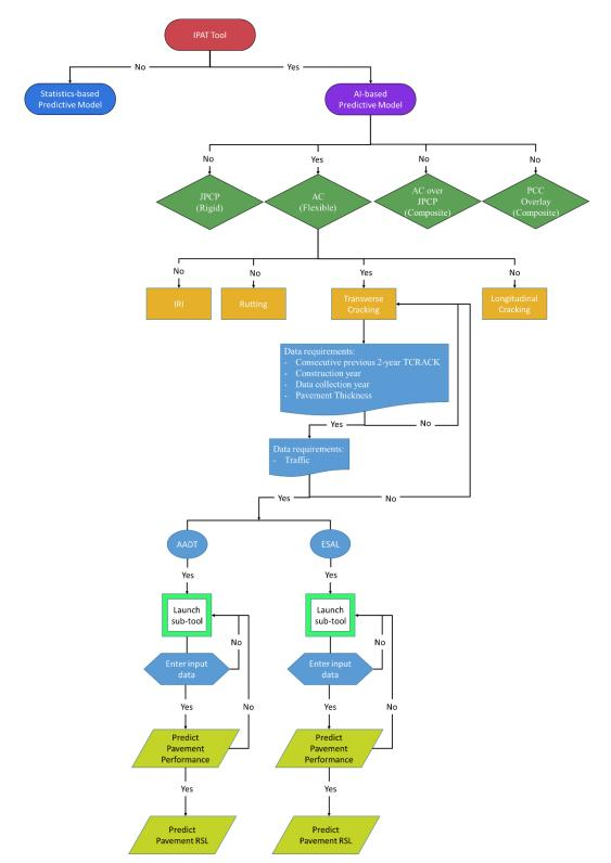
Figure 13. Flowchart of IPAT tool using AI-based TCRACK model for AC
