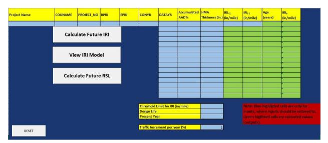
Figure 23. Sub-tool to predict IRI using AI-based IRI approach 1 county model for AC (launch tool 1 in main tool)
