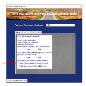
Figure 53. Select pavement performance indicator and prepare data: IRI (AI-based model)
