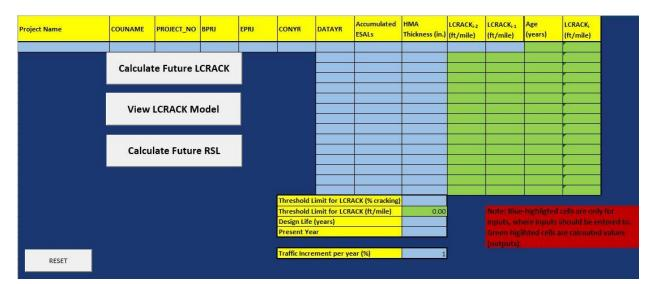
Figure 31. Sub-tool to predict LCRACK using AI-based PMIS model for AC (launch tool 2 in main tool)
