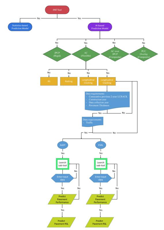
Figure 14. Flowchart of IPAT tool using AI-based LCRACK model for AC
