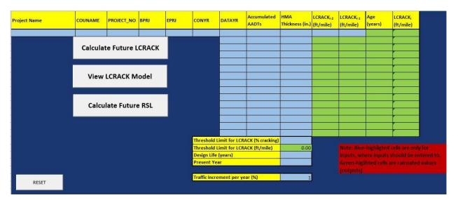
Figure 30. Sub-tool to predict LCRACK using AI-based county model for AC (launch tool 1 in main tool)
