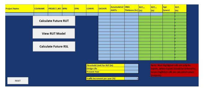
Figure 26. Sub-tool to predict RUT using AI-based county model for AC (launch tool 1 in main tool)
