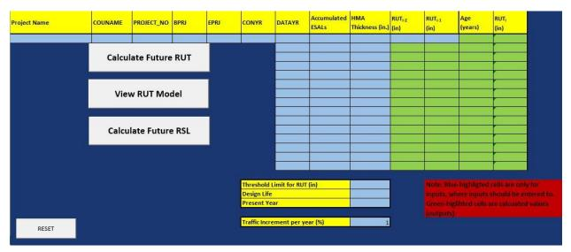
Figure 34. Sub-tool to predict RUT using AI-based PMIS model for AC over JPCP
