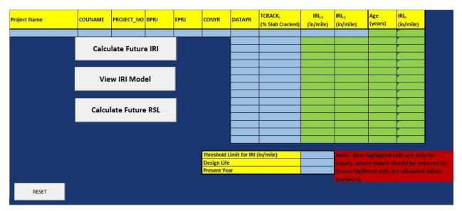
Figure 20. Sub-tool to predict IRI using AI-based IRI approach 2 PMIS model for JPCPs (launch tool 4 in main tool)
