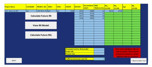
Figure 79. Option 1: Enter existing input parameters and traffic increment per year: AC (AI-based model)
