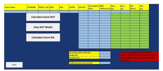
Figure 27. Sub-tool to predict RUT using AI-based PMIS model for AC (launch tool 2 in main tool)
