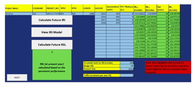
Figure 63. Threshold limit for IRI (130 in./mi), design life (40 years), and present year (2021): JPCP (AI-based model)
