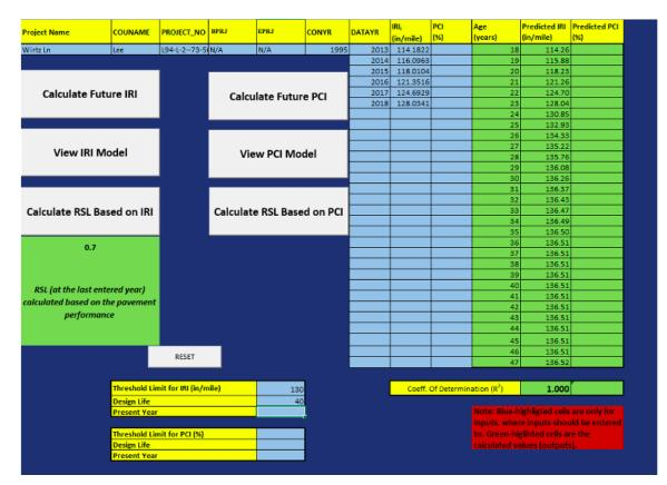
Figure 50. Threshold limit for IRI (130 in./mi) and design life (40 years): JPCP (statisticsbased model)
