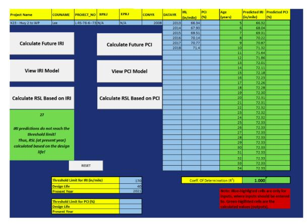
Figure 72. Threshold limit for IRI (170 in./mi), design life (40 years), and present year (2021): AC (statistics-based model)
