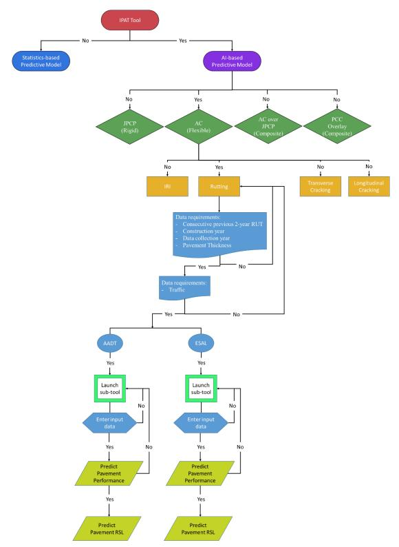
Figure 12. Flowchart of IPAT tool using AI-based RUT model for AC
