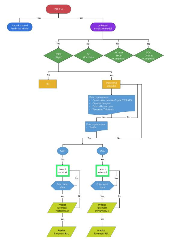
Figure 10. Flowchart of IPAT tool using AI-based TCRACK model for JPCP
