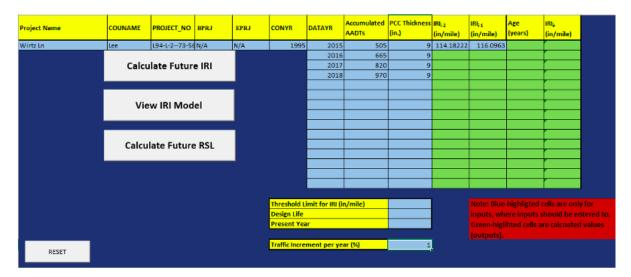
Figure 56. Option 1: Enter existing input parameters and traffic increment per year: JPCP (AI-based model)
