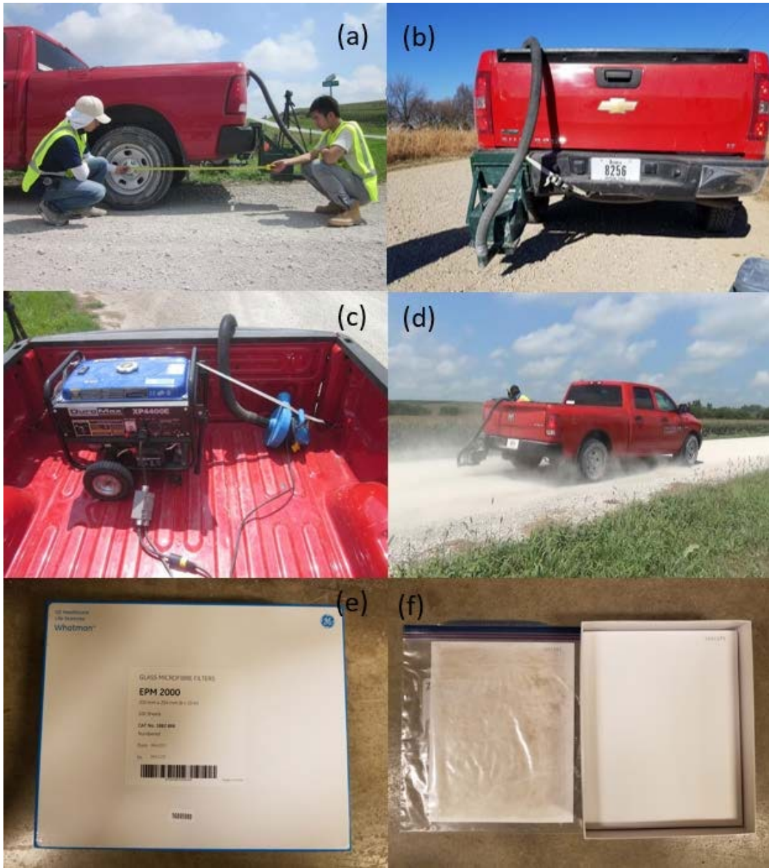
Figure 13. (a, b, and c) Dustometer test setup, (d) test conducted on a granular-surfaced road test section, (e) EPM 2000 glass microfibre filters, and (f) filter sheet before and after a test
