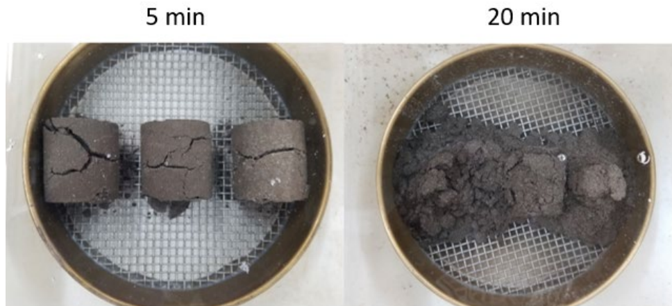
Figure 7. Slaking test for 2 \times 2 specimens of existing surface aggregates from Washington County mixed with 7% clay slurry by dry weight
