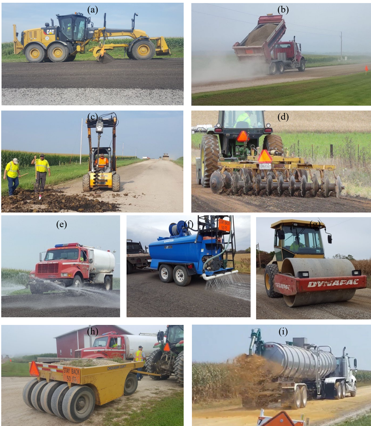
Figure 20. Equipment used for construction of mechanically stabilized sections: (a) motor grader, (b) dump truck, (c) power auger, (d) disc plow harrow (Cherokee County), (e) water truck, (f) water trailer (Cherokee County), (g) smooth drum vibratory compactor, (h) rubber tire roller, and (i) self-unloading tanker trailer
