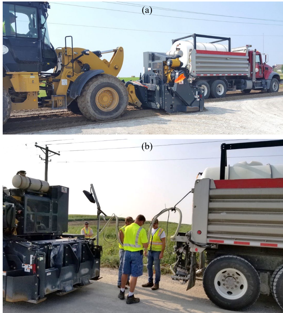
Figure 37. (a) RoadHog milling machine mounted on wheel loader and (b) hose connection to water truck
