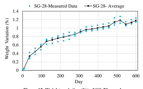
Figure 12. Weight variation (%) of SG-28 samples
