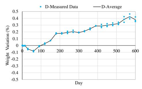
Figure 10. Weight variation (%) of samples with damaged painted galvanized coating
