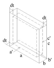
Figure 6. Coupon sample dimensions before and after corrosion
