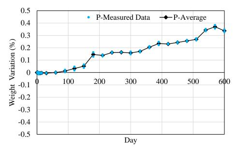
Figure 9, Weight variation (%) of samples with painted galvanized coating
