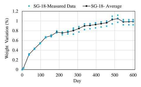
Figure 11. Weight variation (%) of SG-18 samples
