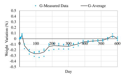
Figure 8. Weight variation (%) of samples with galvanized coating
