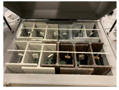
Figure 4. Samples inside the cyclic corrosion chamber
