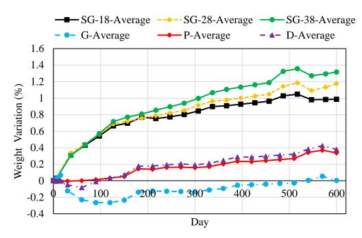
Figure 16. Comparison of average weight variation (%) for G, P, D, and SG samples
