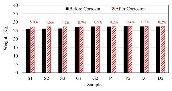
Figure 14. Weight variation in one-foot pile sections
