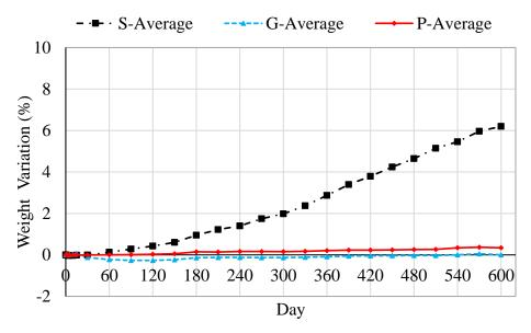
Figure 15. Comparison of average weight variation (%) for S, G, and P samples
