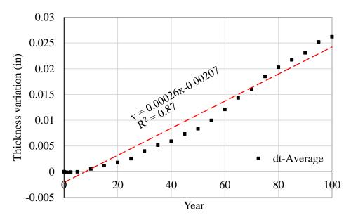
Figure 7. Estimated thickness loss of the bare steel in each year
