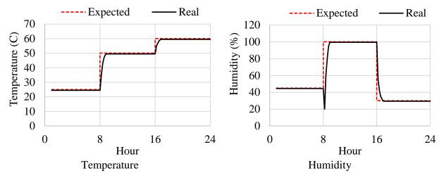
Figure 3. Temperature and humidity variation during each cycle
