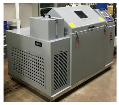
Figure 2. Cyclic corrosion test chamber
