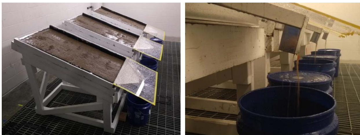
Figure 21. Typical rainfall simulation and captured sediment-laden water runoff
