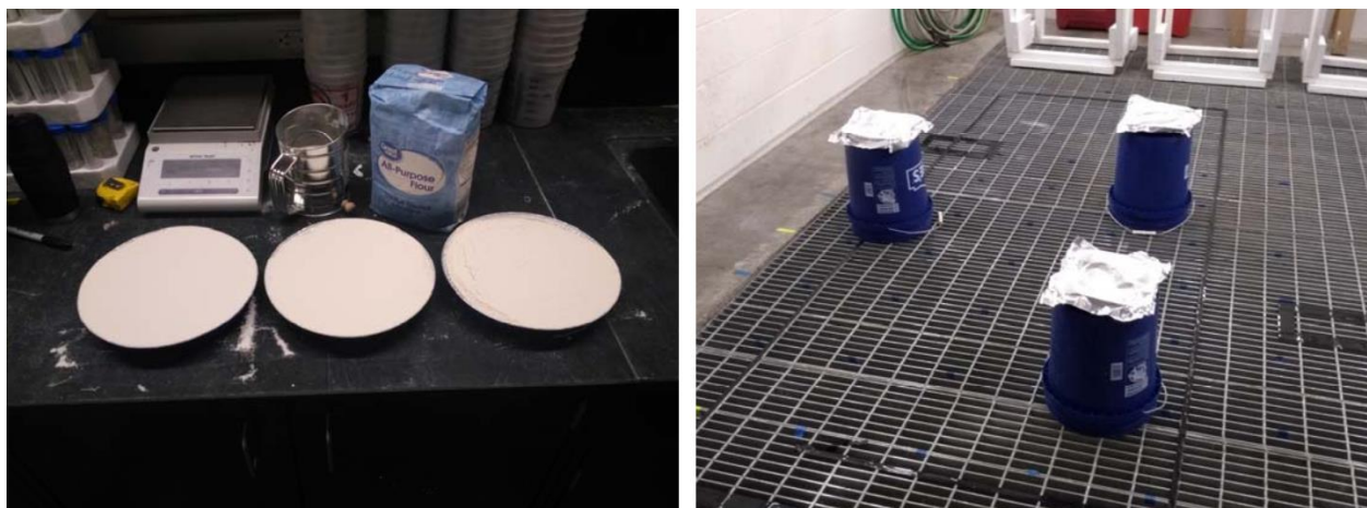
Figure 19. Raindrop particle size distribution test (flour test)
