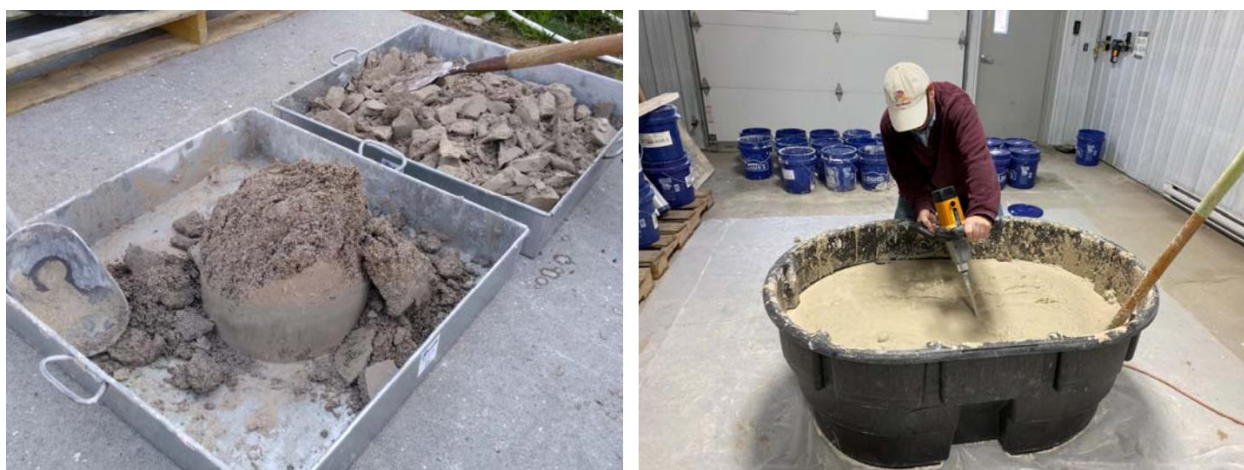
Figure 4. Typical CGR cakes (left) and CGR slurry mixing process (right)
