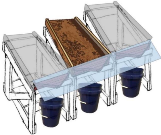
Figure 10. Conceptual design sketch (left) and completed (built) version of rainfall test apparatus (right)
