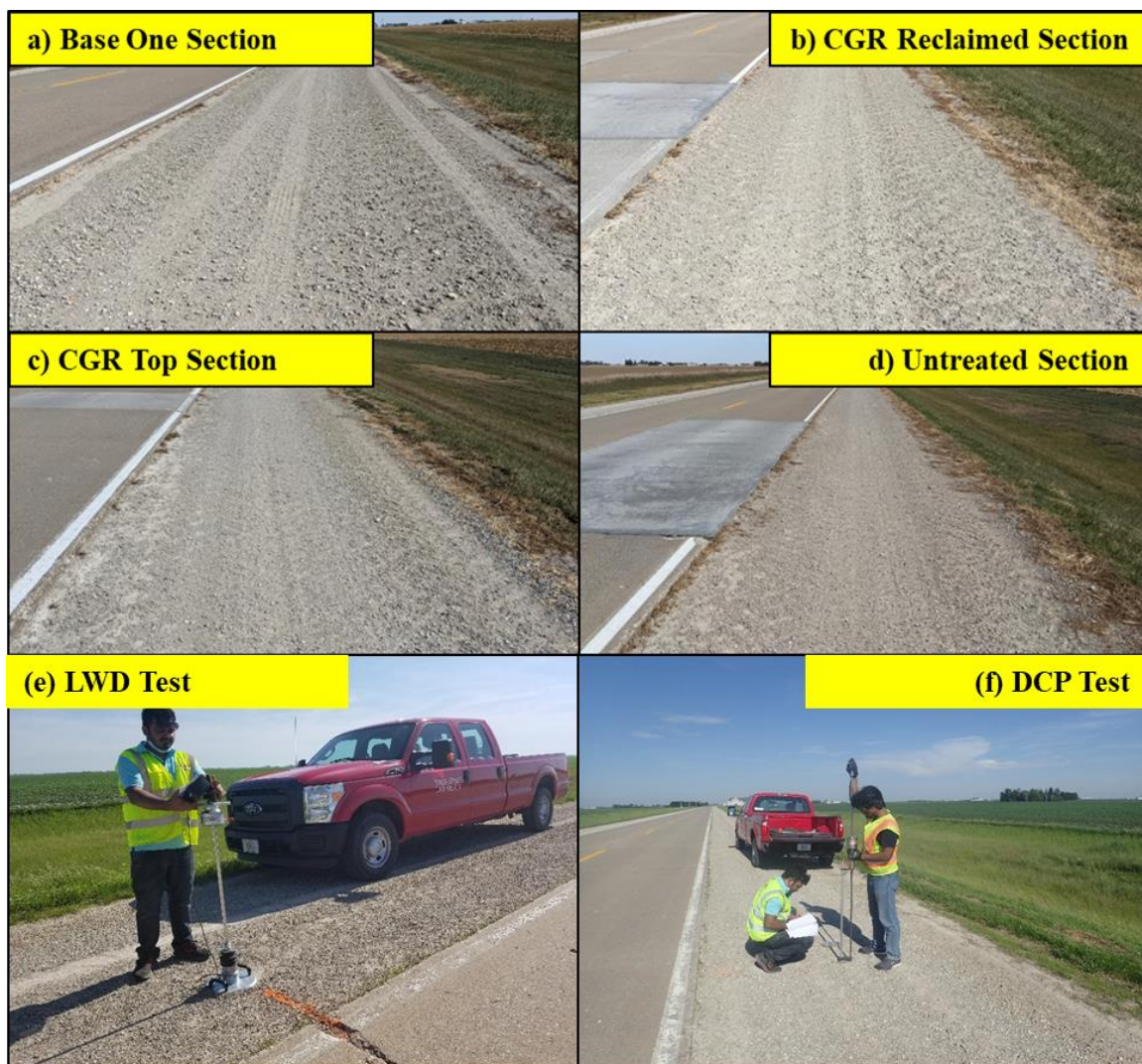
Figure 54. Washington County site appearance after two years: (a) Base One-treated section, (b) CGR Reclaimed section, (c) CGR Top section, (d) untreated section, (e) LWD testing, and (f) DCP testing
