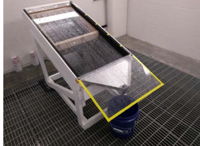
Figure 10. Conceptual design sketch (left) and completed (built) version of rainfall test apparatus (right)
