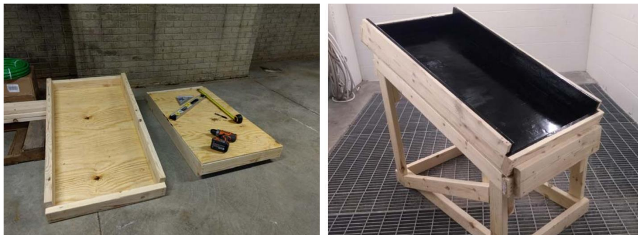
Figure 9. Construction of wooden rainfall soil forms (left) and supporting rack (right)
