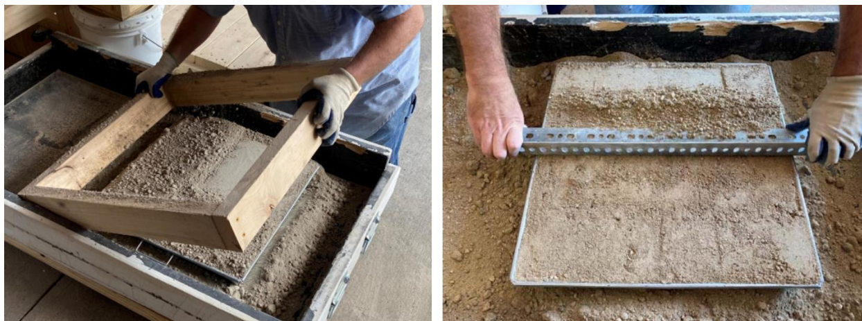
Figure 37. Preparation and screeding of compacted soil form
