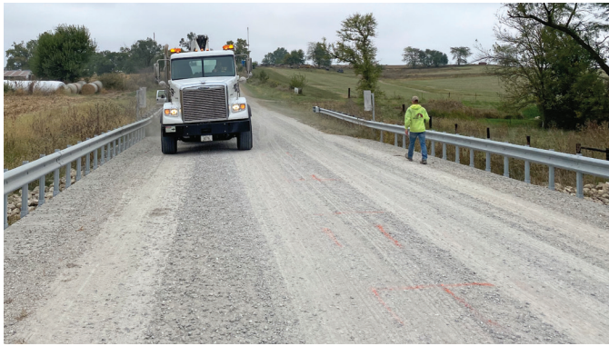
Live load testing
