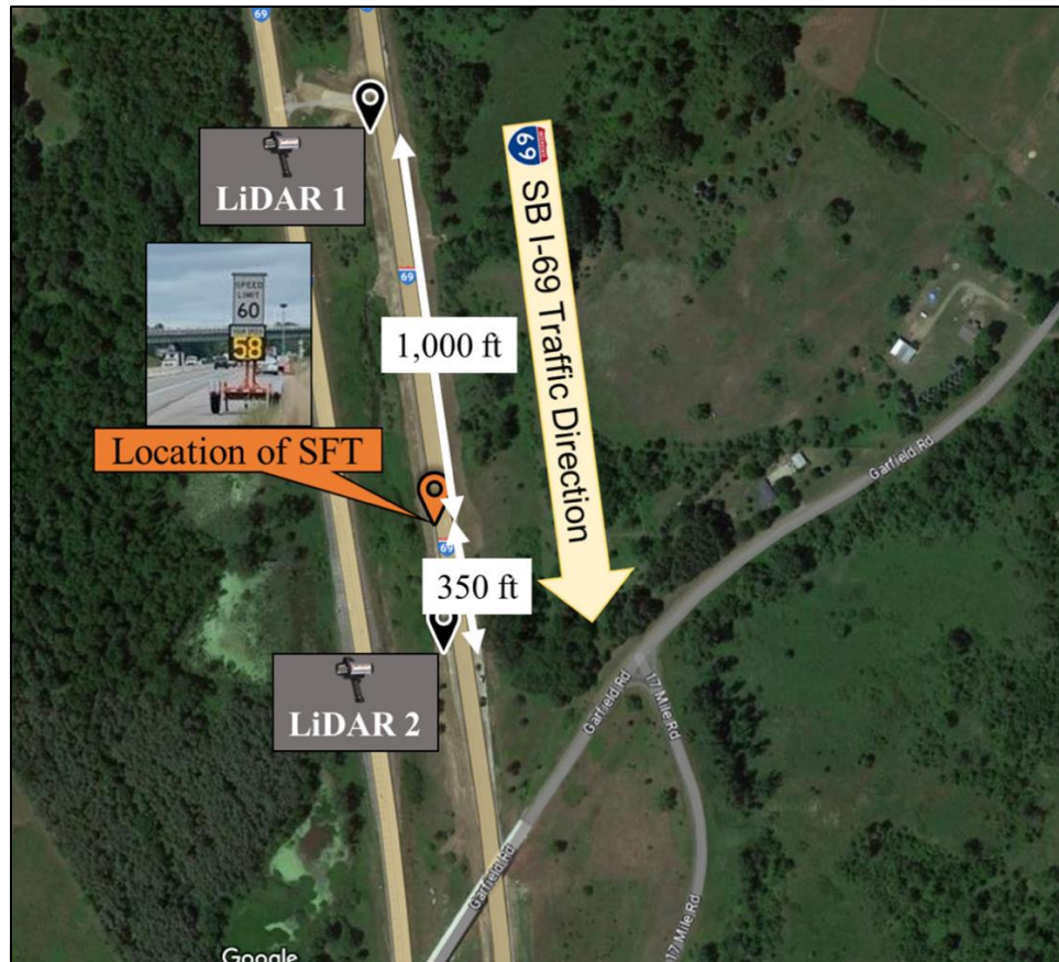
Figure 35. Data collection setup at the work zone study site, SB I-69, Olivet, Michigan
