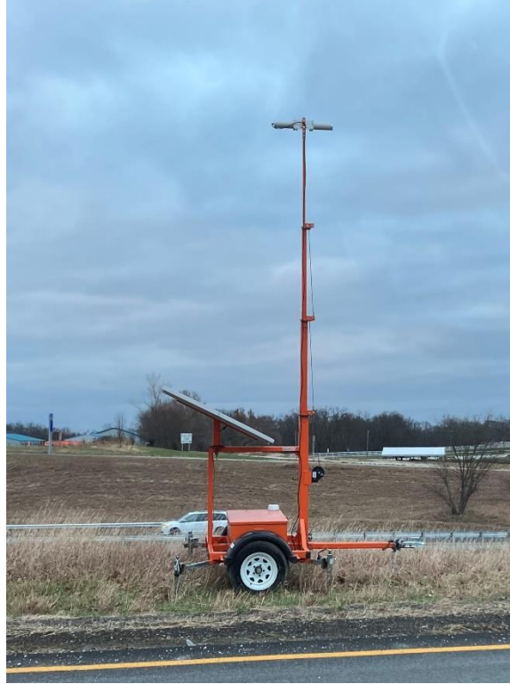
Figure 18. Speed sensor mounted on portable trailer at upstream location (eastbound entrance ramp of the I-70 interchange at MO-179)
