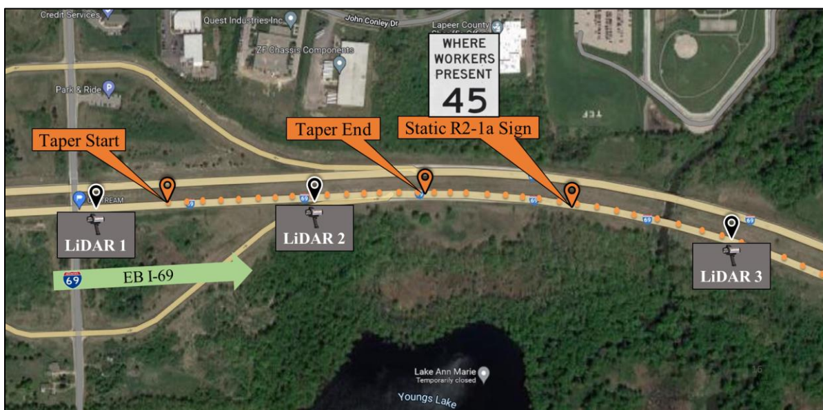
Figure 12. Eastbound I-69 work zone study site layout to evaluate optimal SFT position near the start of the freeway work zone lane closure
