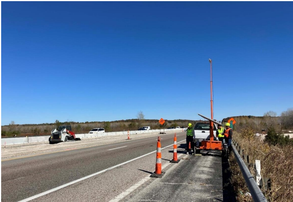
Figure 19. Speed sensor mounted on portable trailer at downstream location (eastbound I-70 near mile marker 113.80)
