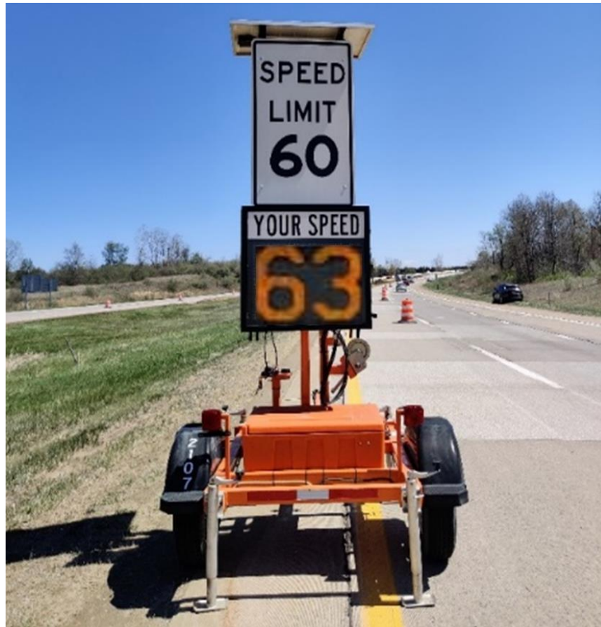
Figure 1. Typical speed feedback trailer used in freeway work zones in Michigan
