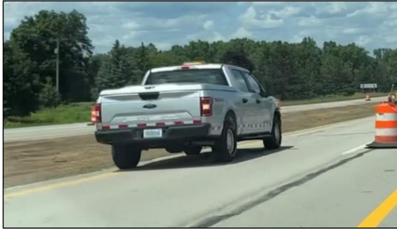
Figure 37. MDOT vehicle (with top beacon and flashers on) positioned at the closed left lane of the Northbound US 127 evaluation site
