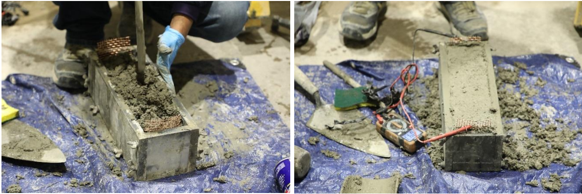
Figure 5. ECON sample collection from ready mixed concrete plant trials
