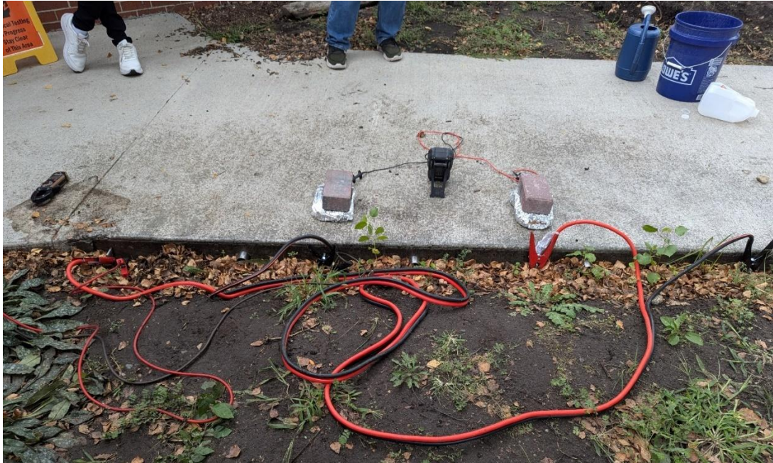
Figure 26. Surface voltage measurement on the ECON demonstration sidewalk site
