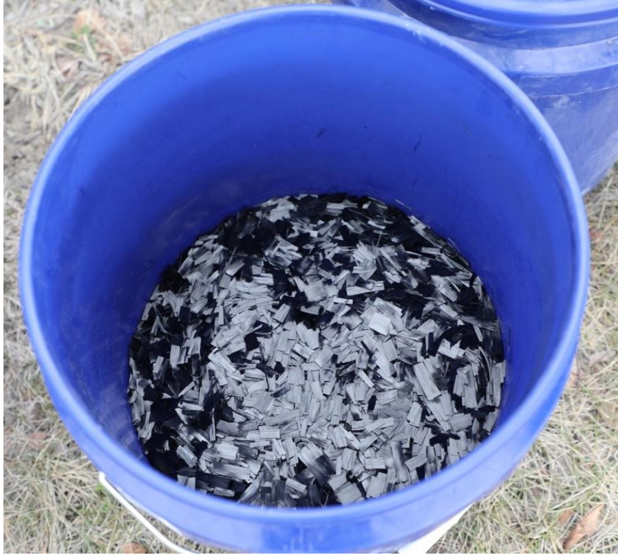
Figure 1. Zoltek corporation PX35 chopped virgin carbon fiber
