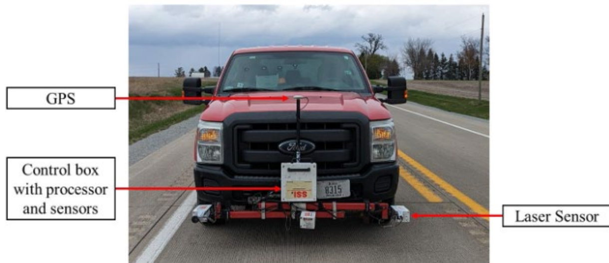
Figure 10. Truck-mounted high-speed profiler system
